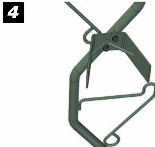
3. Insert the remaining Stick Section (item A) together by inserting the swaged end into the open bottom end. Ensure all stand-offs are aligned. *See figure 3 and 4.*
